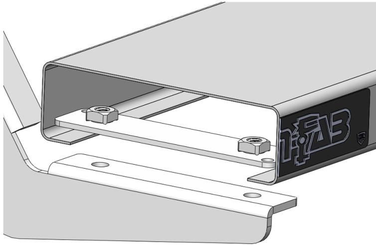
**Step 9:** After final adjustment, tighten all running board threaded mounts.
