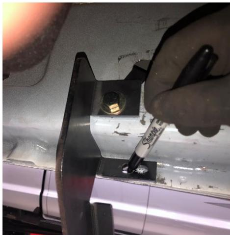
**Step 5:** Install the (x3) rocker panel mounting brackets to the factory attachment points using the provided 3/8" x 1" hex bolts and 3/8" flat washers for the upper mount and the M8x25mm flanged bolt and M8 flanged nut for the pinch weld mount. Leave loose for now.
