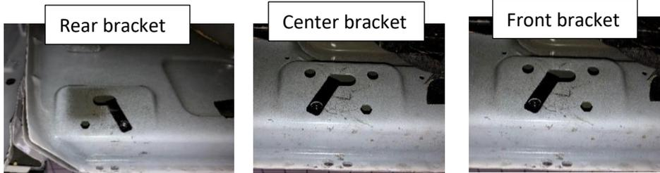
U-clip positioning. **NOTE:** U- Clip orientation will be the same for passenger
